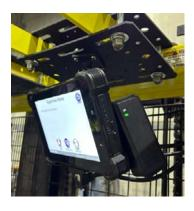
The display should be in a location where both the reader and touch screen display is easily accessible and available to the operator.
