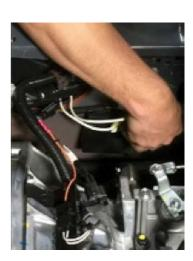
Cabling must be secured and routed in a way that it is free from excessive heat, moving components, and high electrical interference areas.
