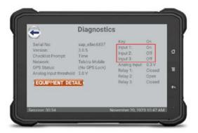
Since there is a change from ON to OFF, jumping off the seat will trigger the change from OFF to ON. GemOne will need to be notified of the direction of the switch (5V to 0V or 0V to 5V) so the correct configuration can be made on the portal.
