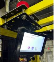
Strobe/Alarm should be positioned to maximise visibility to the operator and surroundings.
