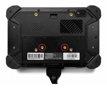
Align the RFID bracket onto the display using the holes highlighted below.
