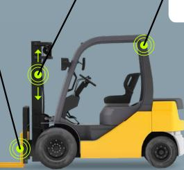
The cameras **automatically record video** to capture data that assists incident investigation.
