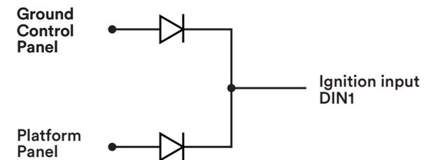
Make sure you use suitable diodes for your application (maximum voltage, ...). Commonly used diode types are: 1N4005 or 1N4007
