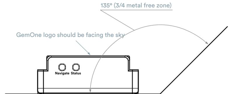
It is not important in which direction the tracker is installed. The most important instruction is that the GSM and GNSS antenna have a good open view.
