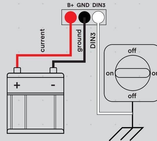
To detect this situation, the tracker needs an additional connection (DIN3 - white) to the chassis. This input can detect invalid signals and will allow the cloud platform to filter other invalid inputs as well. Make sure you enable input filtering in the cloud platform on digital input 3 when this feature is needed.
