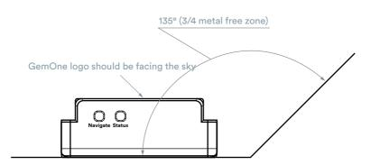
It is not important in which direction the tracker is installed. The most important instruction is that the GSM and GNSS antenna have a good open view.
