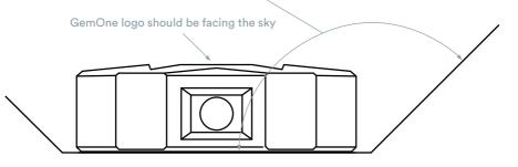
It is not important in which direction the tracker is installed. The most important instruction is that the GSM and GNSS antenna have a good open view.
