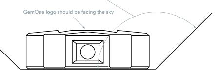
It is not important in which direction the tracker is installed. The most important instruction is that the GSM and GNSS antenna have a good open view.
