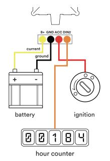
B+, GND and ACC (DIN1) are mandatory for every installation.
