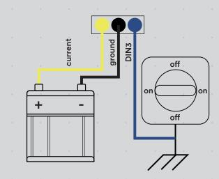
To detect this situation, the tracker needs an additional connection (DIN3 - blue) to the chassis. This input can detect invalid signals and will allow the cloud platform to filter other invalid inputs as well. Make sure you enable input filtering in the cloud platform on digital input 3 when this feature is needed.
